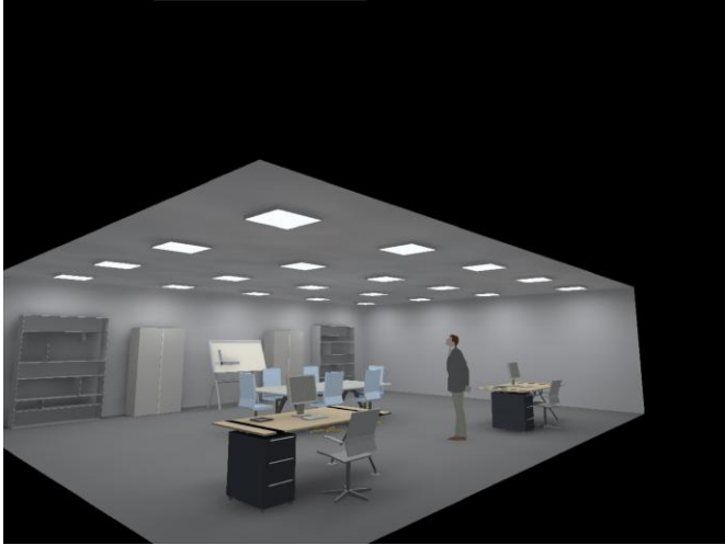
Office view with applying luminaires and their light distribution around the room.
