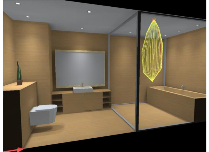
Bathroom view with light distribution curves
