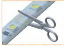
Cut the LED strip in cutting points
