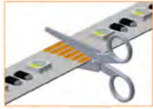
Cut the LED strip in cutting points
