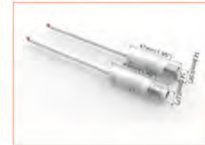
IP67 Connector 2PIN Order Code: AD007-2 Wire Gauge: 0.519mm 2 /20AWG Protection: IP67 (Mated) Mechanical Operation: >500 mating cycles
