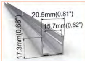
Aluminium Profile Order Code: AC033-AP Dimension: 1000x20.5x17.6mm/ 39.37"x0.81"x0.69"(LxWxH) Material: aluminium Color: silver
