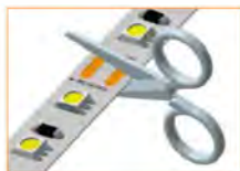
Cut the LED strip in cutting points
