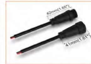
IP67 Connector 2PIN Order Code: AD024-2 Wire Gauge: 0.519mm 2 /20AWG Protection: IP67 (Mated) Mechanical Operation: >500 mating cycles
