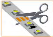
Cut the LED strip in cutting points
