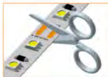
Cut the LED strip in cutting points
