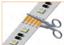
Cut the LED strip in cutting points
