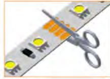
Cut the LED strip in cutting points
